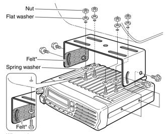
When using self-tapping screws
