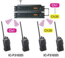
The IC-F3102D series can be used in an IDAS single-site trunking system.
