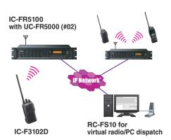
When using the IC-F3102D series in IDAS multi-site conventional mode, the IC-F3102D can communicate with other IDAS radio users working with other repeater sites and/or virtual radio/PC dispatch stations on the IDAS network.
