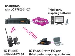
When used with the optional GPS speakermicrophone, HM-171GP, the IC-F3102D series can transmit accurate position data to other advanced IDAS radios and/ or connected PC for use with vehicle management applications.
