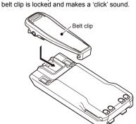
• Lift the tab up (1), and slide the belt clip in the direction of the arrow (2).
